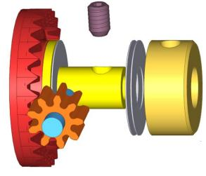
This is what happens, when it happens: the areas in red, when the oil film breaks, are in contact with each other and lap after lap start slowing your car down as the surface wear takes place. A grinding noise may be heard and bronze or aluminium brass may be found. The process is not reversible.
